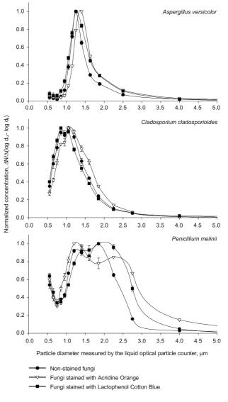
Figure 4. Size distribution of three different fungi determined by a light scattering spectrometer with and without microbiological stains applied.
