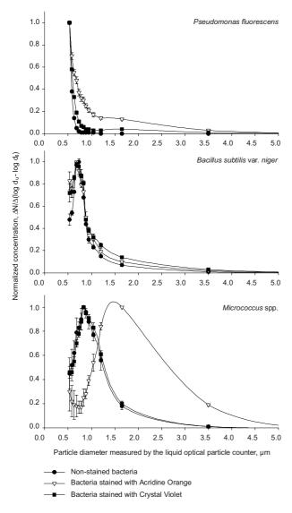
Figure 3. Size distribution of three different bacteria determined by a light scattering spectrometer with and without microbiological stains applied.
