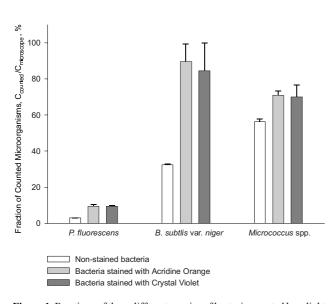
Figure 1. Fractions of three different species of bacteria counted by a light scattering spectrometer with and without stains applied.
